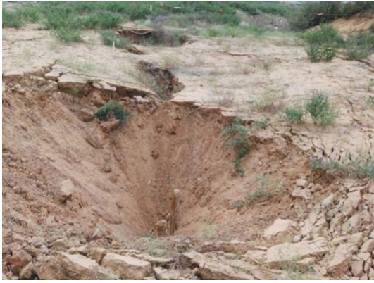
Fig. 3 Site image of ground subsidence due to water and sand inrush from the inclined shaft
